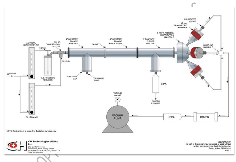
Setup 2: Alternative to ASTM 2299: Tests with Salts or Pedialyte
